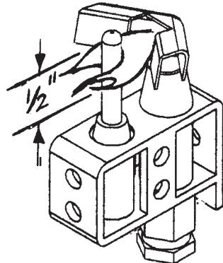
If the closed circuit check shows thermocouple output is greater than 8 millivolts and pilot will not remain lit when reset button is released, replace safety pilot magnet assembly.
