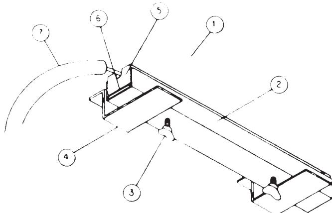
Thermostat sensing bulb holder assembly.
